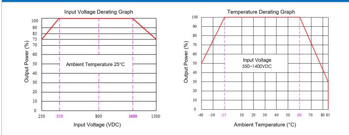
Note 1: The output power should be derated based on the input voltage derating graph at 250~350VDC/1400~1500VDC.
